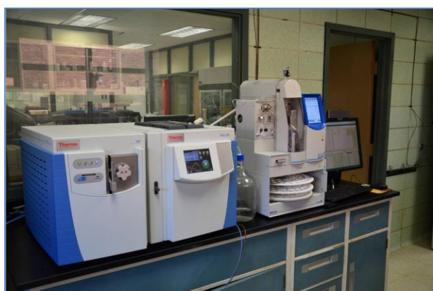
Figure 2. Thermo Gas Chromatograph with Mass Spectrometer Detector (GC/MS) and Organics Detection System Parameters Source: Workshop Presentation by Jerry Schulte, ORSANCO, August 19, 2014.
